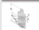
We recommend that separators be used if multiple round cables or conduits with differing diameters are to be installed. An offset configuration of the separators is advisable.
