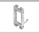
For frame bridges wider than 246 mm, we recommend the use of crossbar connectors. These prevent deformation to the frame bridge under large amounts of additional weight of the chain assembly.
