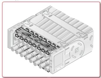
They are secured in much the same way as the frame bridges themselves, by snapping them into pre-cut recesses in the chain brackets. This enables two strain relief plates to be integrated into the cable drag chain per cable end, both for the inside bend and the outside bend.
